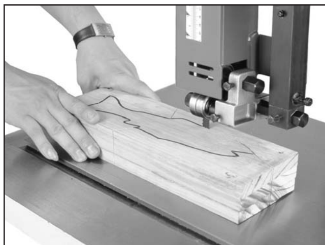
Figure 36. Cutting multiple pieces at once.
